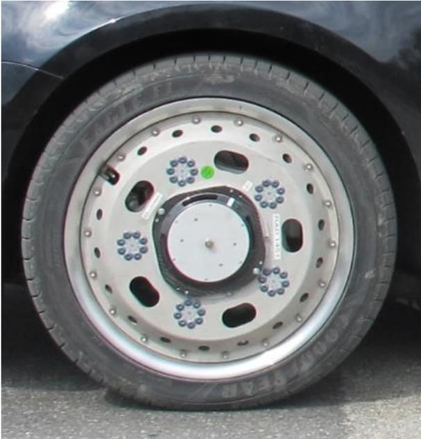
Fig.5 Wheel force transducer
