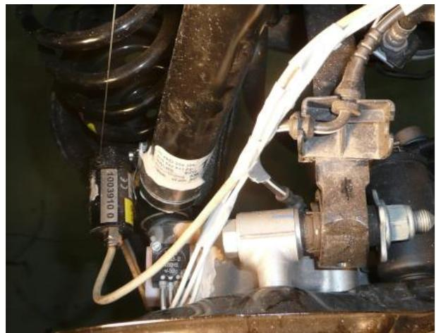
Fig.4 Spring displacement measured by wire based sensor and acceleration sensor
